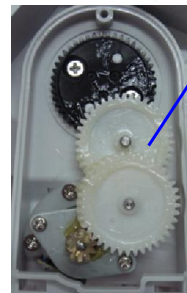
Intricate gear transmission for smooth and quiet operation
